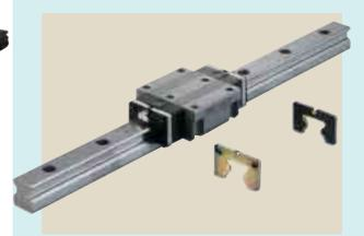
The capillary plate is assembled inside of the end seal in the slide unit. It is impregnated with lubricant so that the re-lubrication interval can be made longer and maintenance time and cost can be saved greatly.
