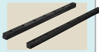
Black chrome surface treatment is a process to form a black permeable film on the slide unit and track rail for corrosion resistance and then apply a protective coating of acrylic resin on top of it.
